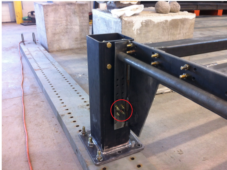
Figure 7.3. Detail of mechanism for modifying the boundary conditions: bolted = fixed; unbolted = pinned.
