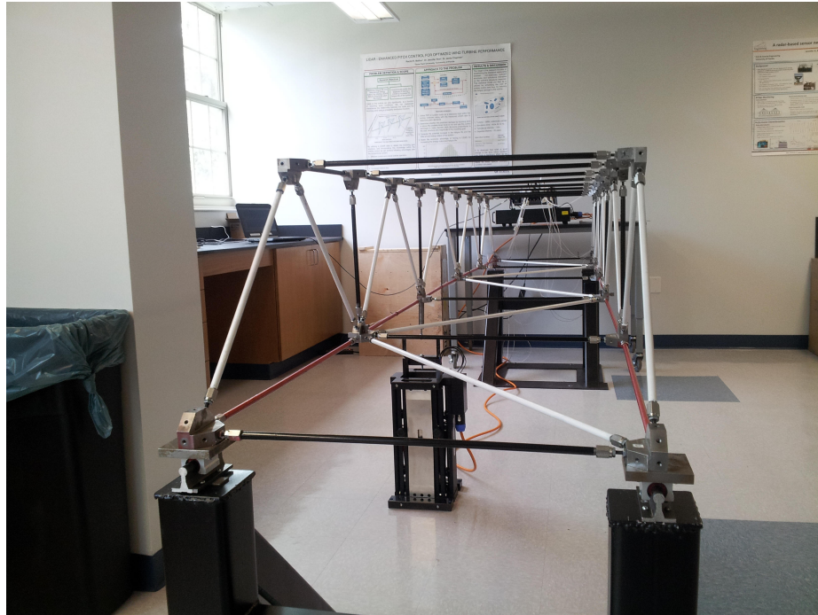
Figure 7.1. Scaled truss bridge for SHM. (Courtesy of Dr. Jennifer A. Rice, University of Florida at Gainesville).
